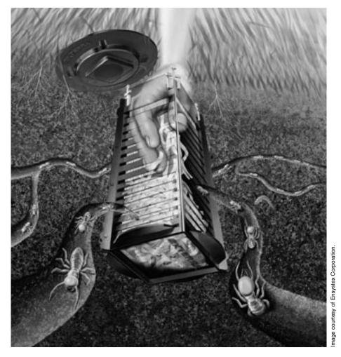
Exterra Termite Inspection and Baiting System, with schematic illustration of termites foraging at the underground station.
